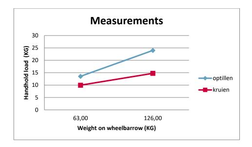
Measured values when barrowing bricks with the Matador brick barrow (average values over 3 measurements).
