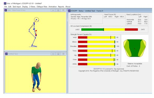
The green area L4/L5 marks the completely safe area for back loading (3415 N value). In the figure this is shown for an average man (175.1 cm and weighing 83.9 KG). The hand forces are 165 Newtons per hand when lifting (because wheelbarrowing is actually lifting), this equals 330 Newtons and this equals a total of 33 KG of force. The yellow area L4/L5 marks the acceptable area for back strain. The red area should be avoided.
